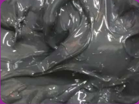
LITHIUM MOLYBDENUM GREASE 3% MOLYBDENUM DISULFIDE
